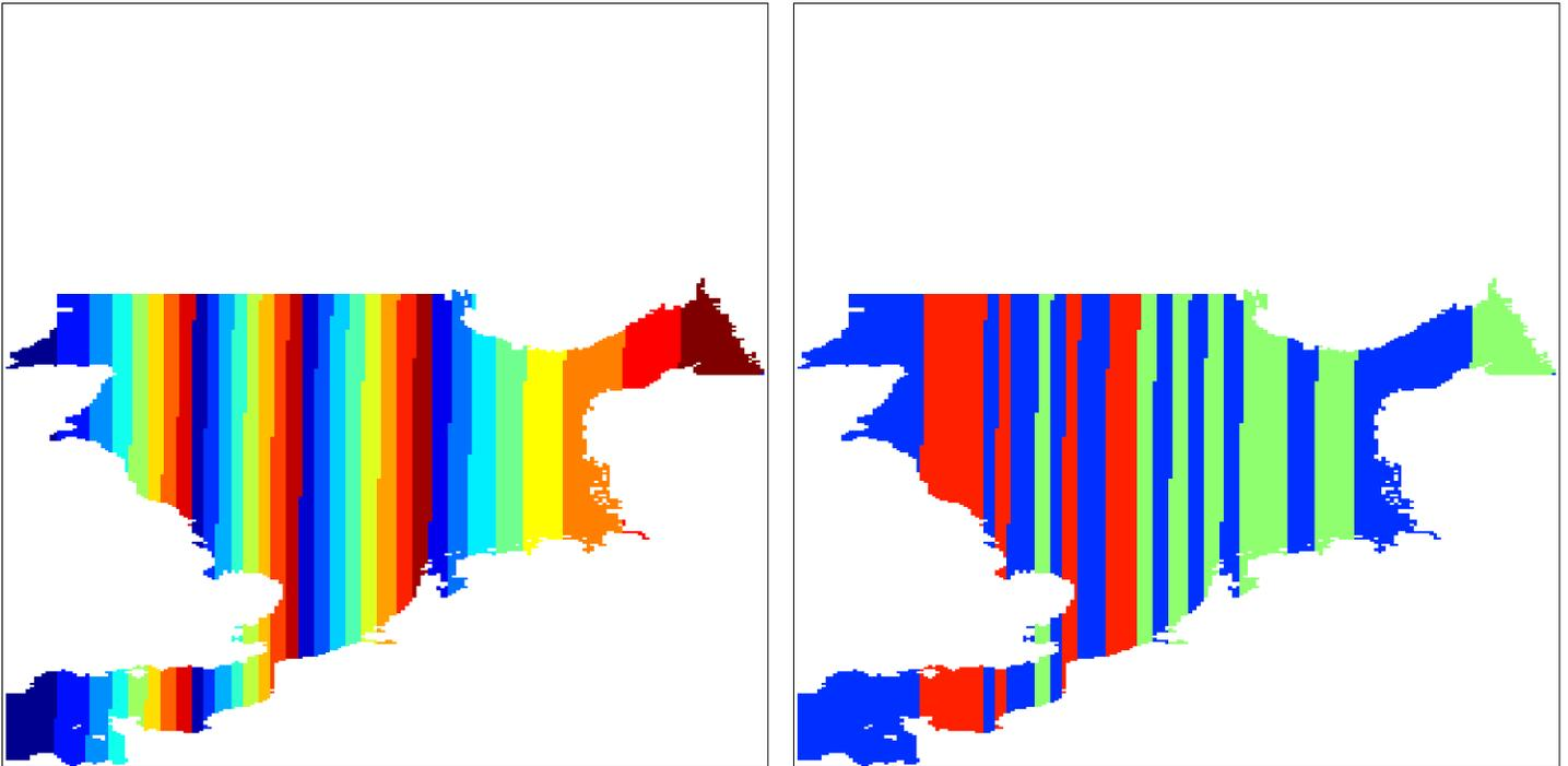
Figure 44: Illustration of the 32 threads openMP decomposition for the North Sea.
