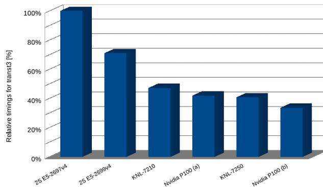
Figure 15. Relative time-to-solution for `transt3` from the best performing code versions on the respective architectures, i.e. this is not portable performance but a result of cross-comparing different versions of the source code, each one explicitly crafted to target an individual architecture. For P100, (a) and (b) are without and with algebraic rewrite of the power function, respectively. The GPU timings do *not* include PCI communication.
