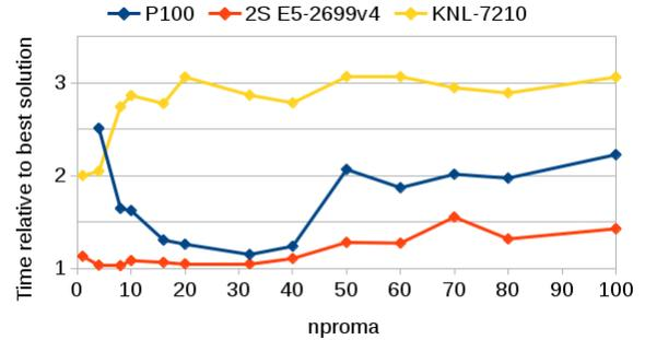
Figure 12. The `nproma` experiment with *time-to-solution* relative to the *time-to-solution* obtained for each of the three platforms with our refactored data organization for varying values of `nproma`. Again, timings are for `transt3`. The GPU timings do *not* include PCI communication.
