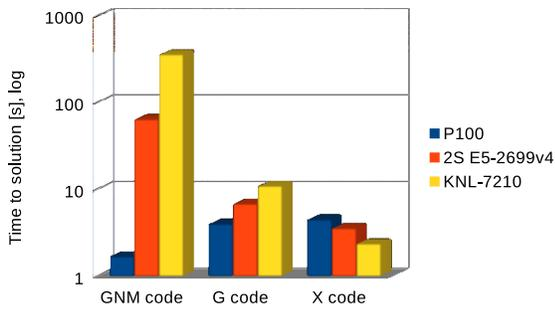
Figure 18. Time-to-solution for the three different code bases on three different architectures. X is the Xeon target code. G is the GPU target code using the data structures as X, but with split into seven chunks. GNM is the GPU target with transposed data structures as compared to X and G, reformulated power function and even more splits (into 12 chunks).
