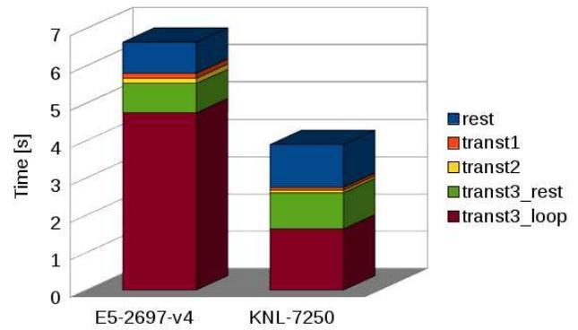
Figure 5. Time-to-solution when running the complete ACRANE2 dwarf on a dual-socket Xeon (72 threads; left) versus single-socket Xeon Phi (272 threads; right). There is almost  $\sim 2x$  difference in the overall performance but there are individual performance differences seen in individual sub-components.
