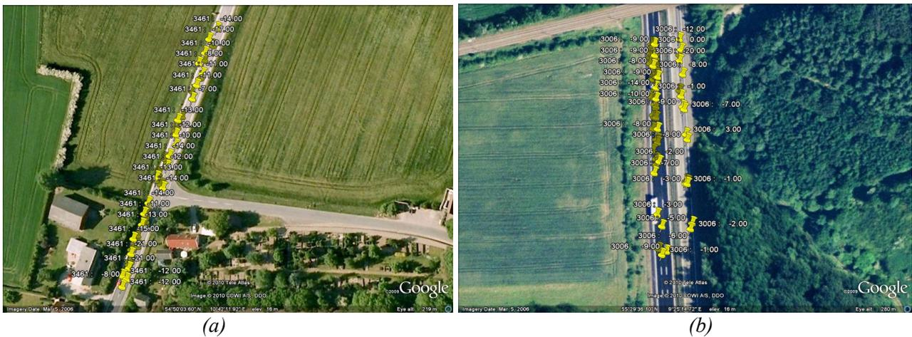
**Figure 3.2.5:** Positions of the ThMD measurements (with highest deviations from the road station measurements) assigned to locations of road stations (a) #3461 and (b) #3006 within a distance interval of  $\pm 75$  meters from the positions of stations (during road season of 2008-2009) /extracted from Google/.
