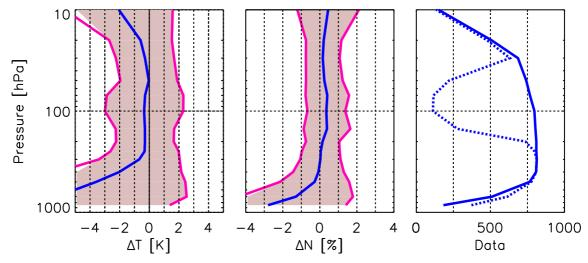
**Figure 4.10**: Comparison (Bias and RMS) of CHAMP dry temperature (left panel) and refractivity (middle) profiles with corresponding RS data (CHAMP-RS) over Australia for May 2001-September 2004 ( $\Delta t = 3~h; d = 300~km$ ). The right panel shows the number of compared data per altitude (solid line: temperature; dashed line: refractivity).
