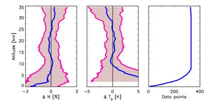
**Figure 4.21**: Comparison (Bias and RMS) of CHAMP refractivity (left panel) and dry temperature (middle) profiles with corresponding ECMWF data (CHAMP-ECMWF) over Japan for May 2001-September 2004 ( $\Delta t=3~h; d=300~km; 331$  profiles).
