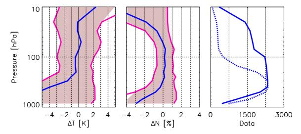
**Figure 4.11**: Comparison (Bias and RMS) of CHAMP dry temperature (left panel) and refractivity (middle) profiles with corresponding RS data (CHAMP-RS) over China for May 2001-September 2004 ( $\Delta t = 3 \ h; d = 300 \ km$ ). The right panel shows the number of compared data per altitude (solid line: temperature; dashed line: refractivity).
