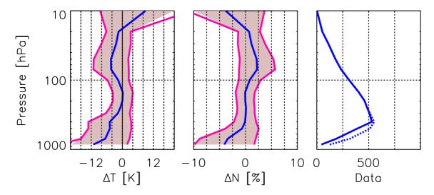
**Figure 4.13**: Comparison (Bias and RMS) of CHAMP dry temperature (left panel) and refractivity (middle) profiles with corresponding RS data (CHAMP-RS) over India for May 2001-September 2004 ( $\Delta t = 3 \ h; d = 300 \ km$ ). The right panel shows the number of compared data per altitude (solid line: temperature; dashed line: refractivity).
