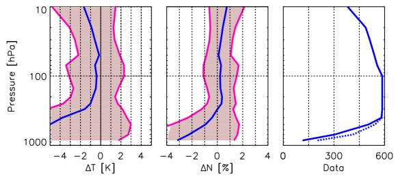
**Figure 4.14**: Comparison (Bias and RMS) of CHAMP dry temperature (left panel) and refractivity (middle) profiles with corresponding RS data (CHAMP-RS) over Japan for May 2001-September 2004 ( $\Delta t = 3~h; d = 300~km$ ). The right panel shows the number of compared data per altitude (solid line: temperature; dashed line: refractivity).
