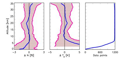
**Figure 4.18**: Comparison (Bias and RMS) of CHAMP refractivity (left panel) and dry temperature (middle) profiles with corresponding ECMWF data (CHAMP-ECMWF) over China for May 2001-September 2004 ( $\Delta t = 3 \ h; d = 300 \ km; 1186 \ profiles).$
