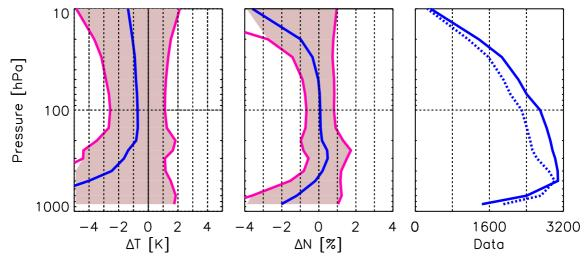
**Figure 4.12**: Comparison (Bias and RMS) of CHAMP dry temperature (left panel) and refractivity (middle) profiles with corresponding RS data (CHAMP-RS) over the countries of the former SU for May 2001-September 2004 ( $\Delta t = 3 \ h; d = 300 \ km$ ). The right panel shows the number of compared data per altitude (solid line: temperature; dashed line: refractivity).
