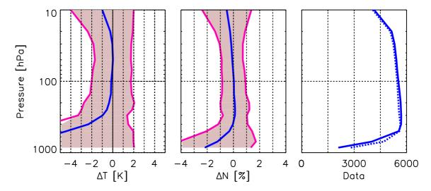
**Figure 4.15**: Comparison (Bias and RMS) of CHAMP dry temperature (left panel) and refractivity (middle) profiles with corresponding RS data (CHAMP-RS) over the U.S. for May 2001-September 2004 ( $\Delta t = 3 \ h; d = 300 \ km$ ). The right panel shows the number of compared data per altitude (solid line: temperature; dashed line: refractivity).
