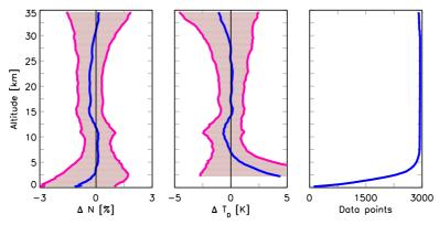
**Figure 4.16**: Comparison (Bias and RMS) of CHAMP refractivity (left panel) and dry temperature (middle) profiles with corresponding ECMWF data (CHAMP-ECMWF) over Europe for May 2001-September 2004 ( $\Delta t = 3 \ h; d = 300 \ km; 2946 \ profiles$ ).
