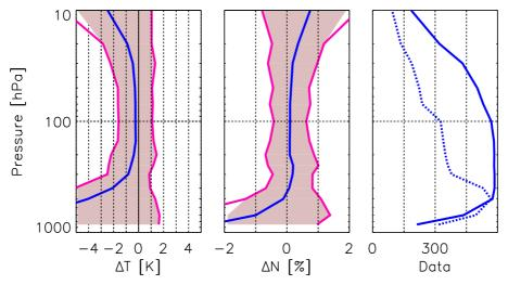
**Figure 4.3**: Comparison (Bias and RMS) of CHAMP dry temperature (left panel) and refractivity (middle) profiles with corresponding RS data (CHAMP-RS) over Europe for May 2001-September 2004 ( $\Delta t = 3~h; d = 100~km$ ). The right panel shows the number of compared data per altitude (solid line: temperature; dashed line: refractivity).
