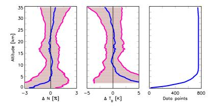
**Figure 4.17**: Comparison (Bias and RMS) of CHAMP refractivity (left panel) and dry temperature (middle) profiles with corresponding ECMWF data (CHAMP-ECMWF) over Australia for May 2001-September 2004 ( $\Delta t = 3~h; d = 300~km; 756$  profiles).
