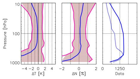
**Figure 4.5**: Comparison (Bias and RMS) of CHAMP dry temperature (left panel) and refractivity (middle) profiles with corresponding RS data (CHAMP-RS) over Europe for May 2001-September 2004 ( $\Delta t = 2 \ h; d = 200 \ km$ ). The right panel shows the number of compared data per altitude (solid line: temperature; dashed line: refractivity).
