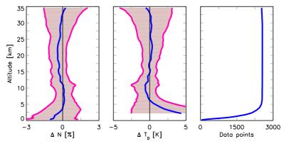
**Figure 4.19**: Comparison (Bias and RMS) of CHAMP refractivity (left panel) and dry temperature (middle) profiles with corresponding ECMWF data (CHAMP-ECMWF) over the countries of the former Soviet Union for May 2001-September 2004 ( $\Delta t = 3 \ h; d = 300 \ km;$  2556 profiles).
