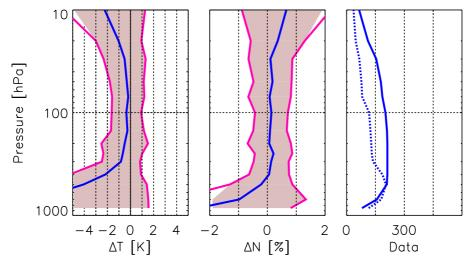
**Figure 4.1**: Comparison (Bias and RMS) of CHAMP dry temperature (left panel) and refractivity (middle) profiles with corresponding RS data (CHAMP-RS) over Europe for May 2001-September 2004 ( $\Delta t = 1 \ h; d = 100 \ km$ ). The right panel shows the number of compared data per altitude (solid line: temperature; dashed line: refractivity).
