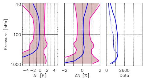
**Figure 4.7**: Comparison (Bias and RMS) of CHAMP dry temperature (left panel) and refractivity (middle) profiles with corresponding RS data (CHAMP-RS) over Europe for May 2001-September 2004 ( $\Delta t = 1 \ h; d = 300 \ km$ ). The right panel shows the number of compared data per altitude (solid line: temperature; dashed line: refractivity).
