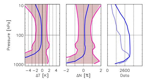
**Figure 4.8**: Comparison (Bias and RMS) of CHAMP dry temperature (left panel) and refractivity (middle) profiles with corresponding RS data (CHAMP-RS) over Europe for May 2001-September 2004 ( $\Delta t = 2~h; d = 300~km$ ). The right panel shows the number of compared data per altitude (solid line: temperature; dashed line: refractivity).
