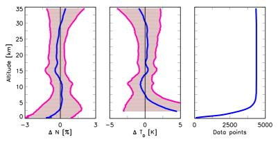
**Figure 4.22**: Comparison (Bias and RMS) of CHAMP refractivity (left panel) and dry temperature (middle) profiles with corresponding ECMWF data (CHAMP-ECMWF) over the U.S. for May 2001-September 2004 ( $\Delta t = 3 \ h; d = 300 \ km; 4372 \ profiles$ ).
