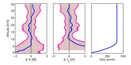
**Figure 4.20**: Comparison (Bias and RMS) of CHAMP refractivity (left panel) and dry temperature (middle) profiles with corresponding ECMWF data (CHAMP-ECMWF) over India for May 2001-September 2004 ( $\Delta t = 3 \ h; d = 300 \ km; 401 \ profiles$ ).
