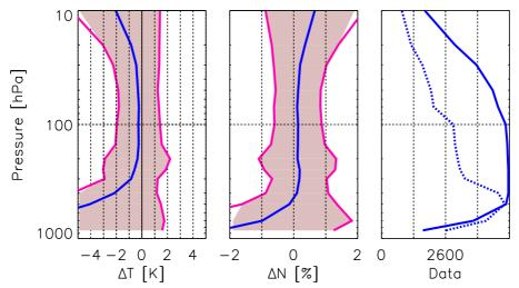
**Figure 4.9**: Comparison (Bias and RMS) of CHAMP dry temperature (left panel) and refractivity (middle) profiles with corresponding RS data (CHAMP-RS) over Europe for May 2001-September 2004 ( $\Delta t = 3 \ h; d = 300 \ km$ ). The right panel shows the number of compared data per altitude (solid line: temperature; dashed line: refractivity).
