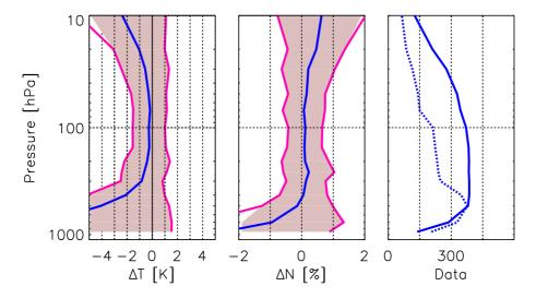
**Figure 4.2**: Comparison (Bias and RMS) of CHAMP dry temperature (left panel) and refractivity (middle) profiles with corresponding RS data (CHAMP-RS) over Europe for May 2001-October 2004 ( $\Delta t = 2~h; d = 100~km$ ). The right panel shows the number of compared data per altitude (solid line: temperature; dashed line: refractivity).
