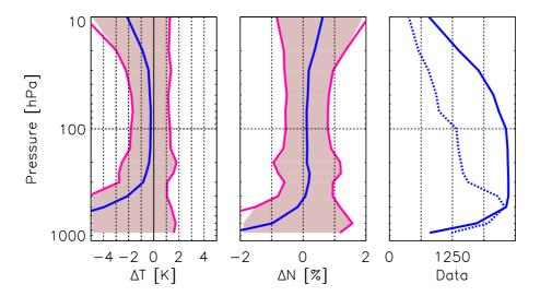
**Figure 4.6**: Comparison (Bias and RMS) of CHAMP dry temperature (left panel) and refractivity (middle) profiles with corresponding RS data (CHAMP-RS) over Europe for May 2001-September 2004 ( $\Delta t = 3 \ h; d = 200 \ km$ ). The right panel shows the number of compared data per altitude (solid line: temperature; dashed line: refractivity).
