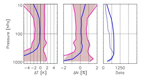
**Figure 4.4**: Comparison (Bias and RMS) of CHAMP dry temperature (left panel) and refractivity (middle) profiles with corresponding RS data (CHAMP-RS) over Europe for May 2001-September 2004 ( $\Delta t = 1 \ h; d = 200 \ km$ ). The right panel shows the number of compared data per altitude (solid line: temperature; dashed line: refractivity).
