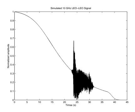
Figure 7-1: Amplitude variations of simulated LEO-LEO signal.
