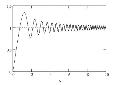
**Figure 4-2:** Solid line: amplitude of chirp integral, CS(x), as a function of x. Dashed line: limiting value of chirp integral,  $|CS(\infty)|$ .
