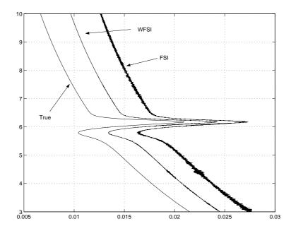
**Figure 7-2:** Noise free signal - comparison between the true bending angle profile and the corresponding profiles retrieved using FSI and WFSI. The FSI and the WFSI profiles are displaced respectively 0.003 radians and 0.006 radians relative to the true profile.
