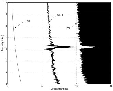
**Figure 7-5:** Noise free signal - comparison between the true profile of optical depth and the corresponding profiles retrieved using FSI and WFSI. The FSI and the WFSI profiles are displaced respectively by 5 and by 10 relative to the true profile.
