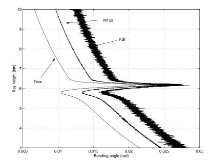
**Figure 7-4:** Noisy signal - comparison between the true bending angle profile and the corresponding profiles retrieved using FSI and WFSI. The FSI and the WFSI profiles are displaced 0.003 radians and 0.006 radians relative to the true profile, respectively.
