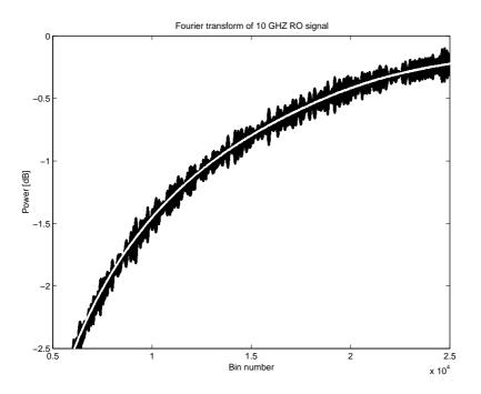
**Figure 5-2:** Comparison between FFT power spectrum, noisy black curve, and power spectrum of the windowed Fourier transform (white curve). The figure is a close-up of Figure 4-1 with the addition of the power spectrum computed using the windowed Fourier transform.
