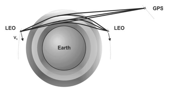
**Figure 1-1:** Principle of combined LEO-LEO and GPS-LEO cross-links. Radio waves emitted by either a LEO or a GPS satellite are received by a LEO satellite setting behind the Earth's limb providing a vertical scan of the atmosphere. The LEO-LEOlinks are sensitive to both ray bending and atmospheric absorption allowing independent observations of water vapor.
