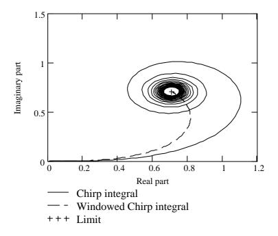
**Figure 4-5:** Same as Figure 4-3 except that results for the windowed chirp integral have been added. Solid curve: Cornu spiral – plotted as real part of chirp integral vs. imaginary part of chirp Integral for  $x \in [0;10]$ . Dashed curve: windowed chirp integral plotted in the same way as the Cornu spiral. Cross: limiting value for  $x \rightarrow \infty$ .
