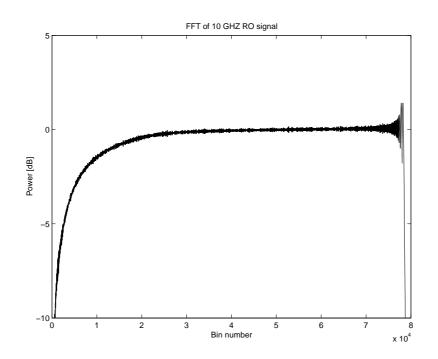
**Figure 4-1:** *Example of FFT of a simulated 10 GHz RO signal with absorption. This power spectrum has both a smooth variation due to atmospheric absorption and rapid oscillations caused by ringing.*
