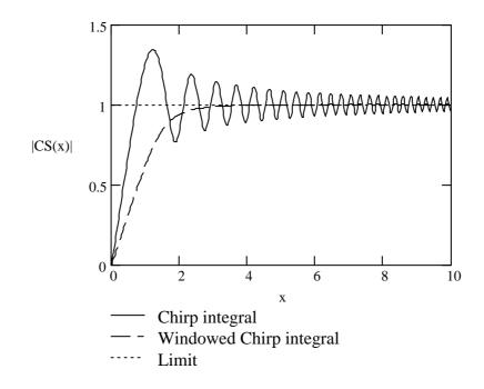
**Figure 4-4:** Same as Figure 4-2 except that results for windowed chirp integral have been added. Solid line: amplitude of chirp integral, CS(x), as a function of x. Dashed line: amplitude of windowed chirp integral  $CS_w(x)$ . Dotted line limiting value of chirp integral,  $|CS(\infty)|$ .
