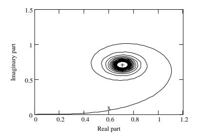
**Figure 4-3:** Solid curve: Cornu spiral – plotted as real part of chirp integral vs. imaginary part of chirp integral for  $x \in [0;10]$ . Cross: limiting value for  $x \rightarrow \infty$ .
