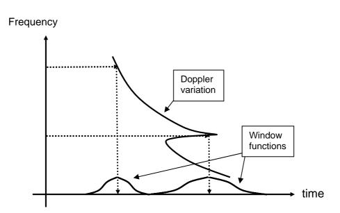
**Figure 5-1:** Principles of windowed FSI: position and durations of window functions are determined for each frequency from the frequency variations predicted by a standard FSI. Long windows are applied when the ray Doppler frequency exhibit slow variations whereas short windows are applied when the ray Doppler frequency has rapid variations.
