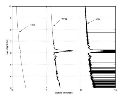
**Figure 7-3:** Noise free signal - comparison between the true profile of optical depth and the corresponding profiles retrieved using FSI and WFSI. The FSI and the WFSI profiles are displaced respectively by 5 and by 10 relative to the true profile.
