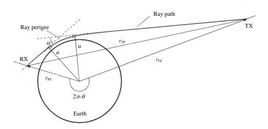
**Figure 2-1:** Geometry of radio occultation. The radio waves propagate from a transmitter, TX, to a receiver, RX, through the Earth's atmosphere.
