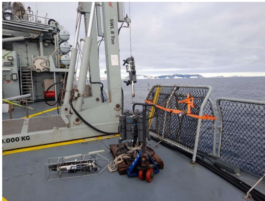
Figure 3: Niskin-Rosette-CTD rack assembled for ICAROS 2021, replacing an integrated SBE911 system planned for the cruise but not mobilized.
