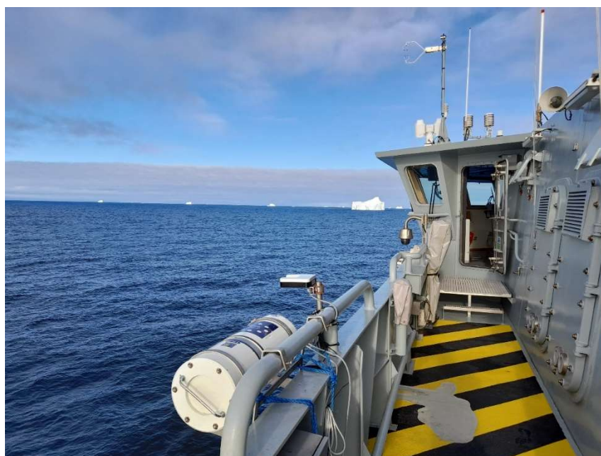
Figure 4: ISAR installation, HDMS Lauge Koch, during ICAROS 2021
