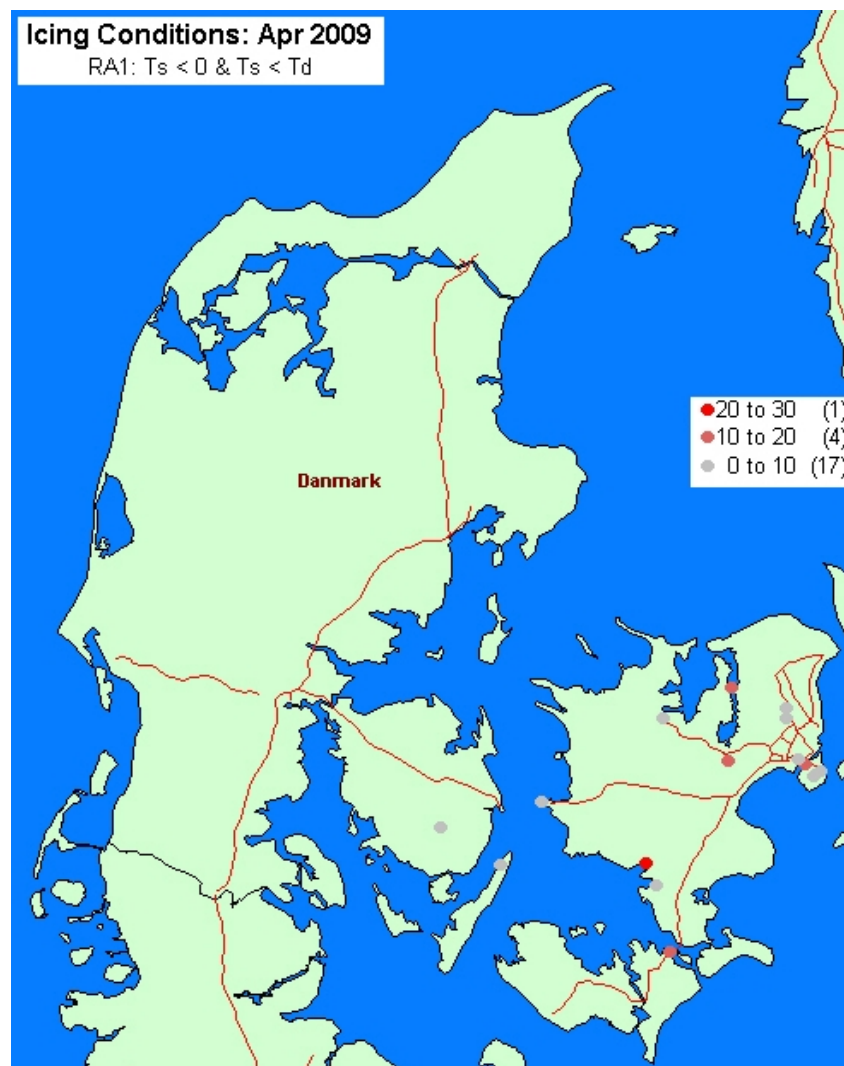
Figure 5D : Spatial distribution of occurrences of the conditions leading to icing on the roads for the red alert situations (RA1) observed at the Danish road stations during April 2009 /number in brackets corresponds to number of the road stations with similar conditions, and intensity of the colored symbol corresponds to higher likelihood of icing/.
