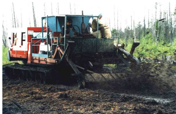
Figure 3-4. 7 years after the oil burnout (left) and ЭМ-2М miller on the base of “Haski” cross-swamp vehicle (right).
