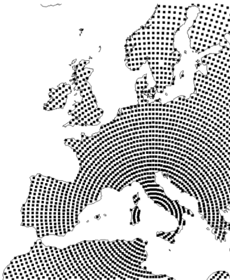
Figure 1: A selection of the model grid points (one black square per grid point) over land and over Europe (the actual model grid covers the whole globe).
