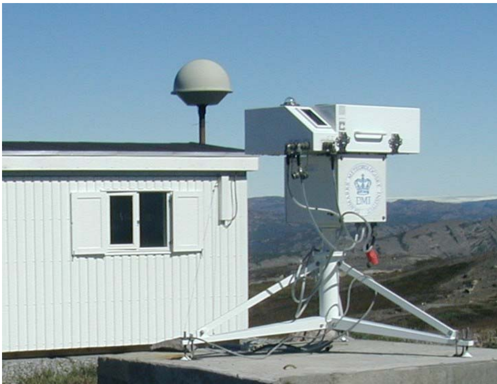
The DMI Brewer spectrometer at Kangerlussuaq, Greenland. The observatories at Kangerlussuaq and Pituffik are part of the Network for Detection of Stratospheric Change (NDSC).
