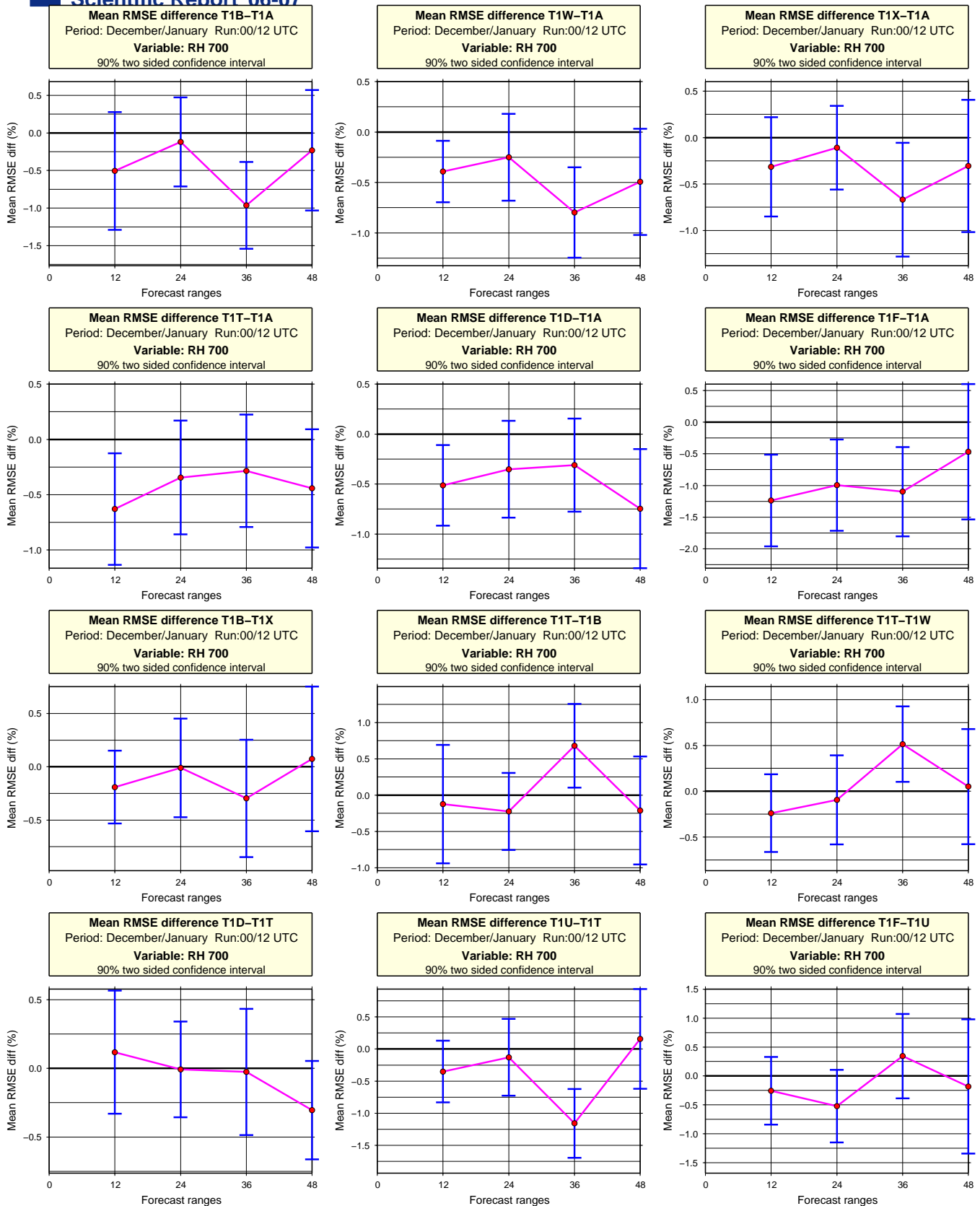
Figure 28: Significance test based on daily scores of 700 hPa relative humidity. 90 % two sided confidence interval. The first model run is better than the second run if the mean is negative. (T1F: all observations used; T1A: baseline run; T1B: T1A + aircraft; T1W: T1A + wind from other radiosondes; T1T: T1A + wind and temperature data from other radiosondes; T1D: T1A + data from all other radiosondes; T1X: T1A + E-AMDAR data; T1V: T1A + wind profiler data; T1U: T1T + all aircraft data)
