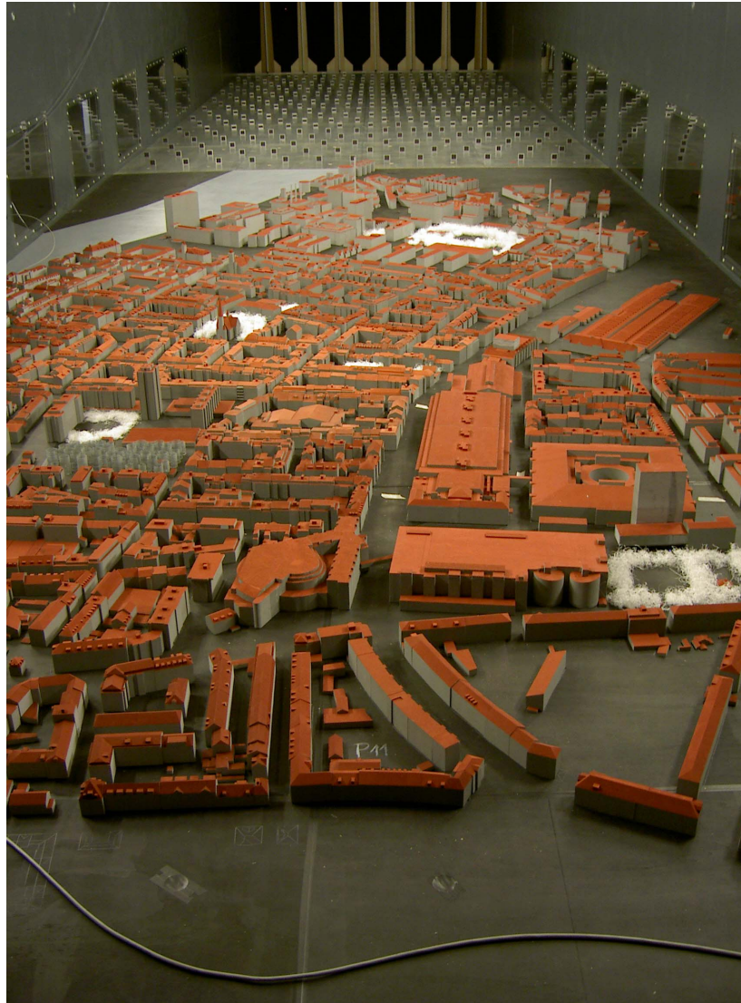
Figure 4.6.1. Model of Basle in MIHU's boundary layer wind tunnel 'WOTAN'. Selected episodes from a field campaign carried out by partner 16 (ETH) will be repeated under controlled ambient conditions.
