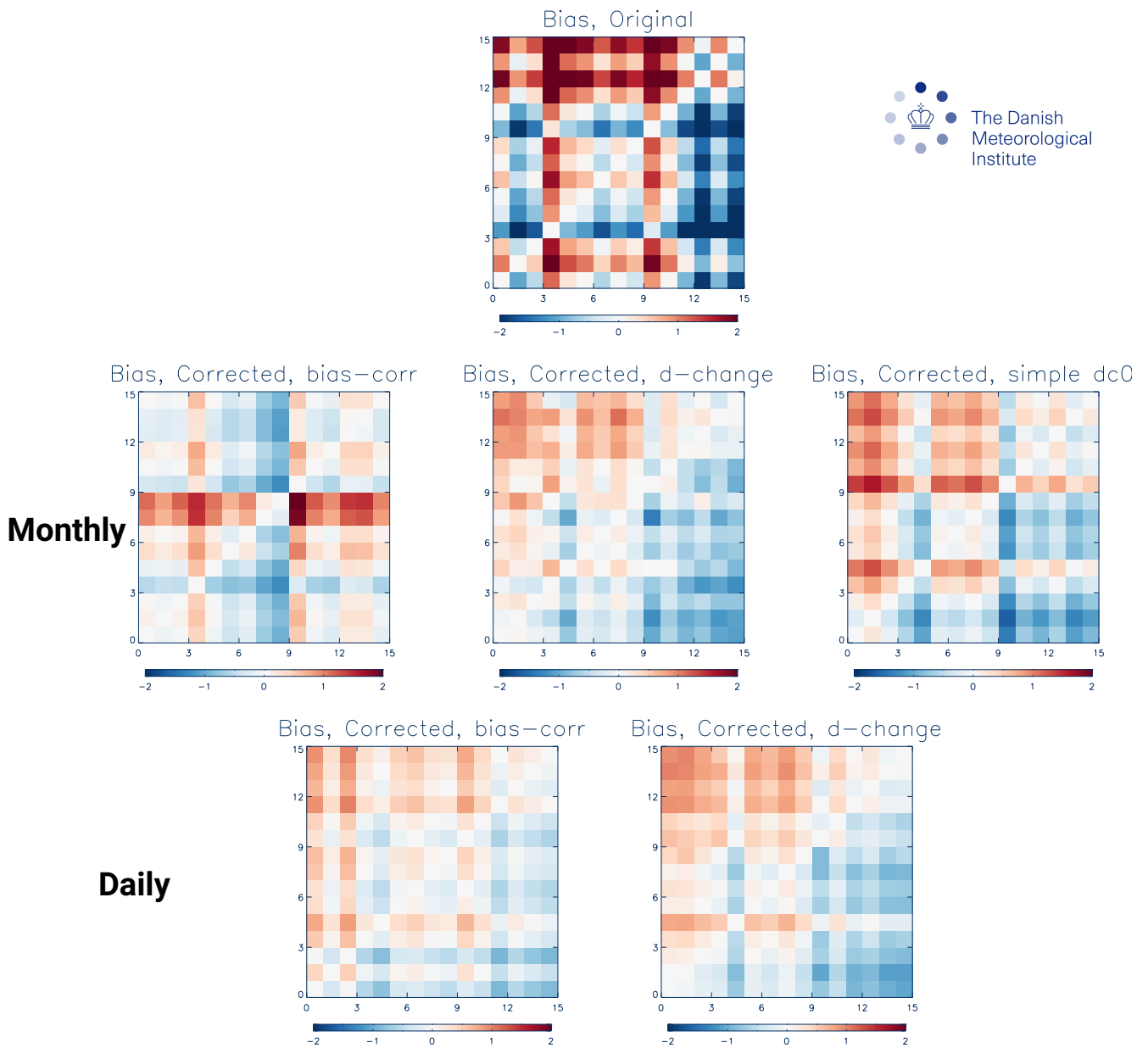
Figure 6: The difference between mean climates in calibrated models and 'truth'. January near-surface temperature. Calibration period 1971-2000, prediction period: 2070-2099. Scenario: RCP8.5. The numbers on the axes refer to the model combinations in Table 2. The horizontal axes indicates the model selected as 'truth'. Top panel shows uncalibrated values. In middle panes calibration is performed on monthly means, in lower panels on daily means.
