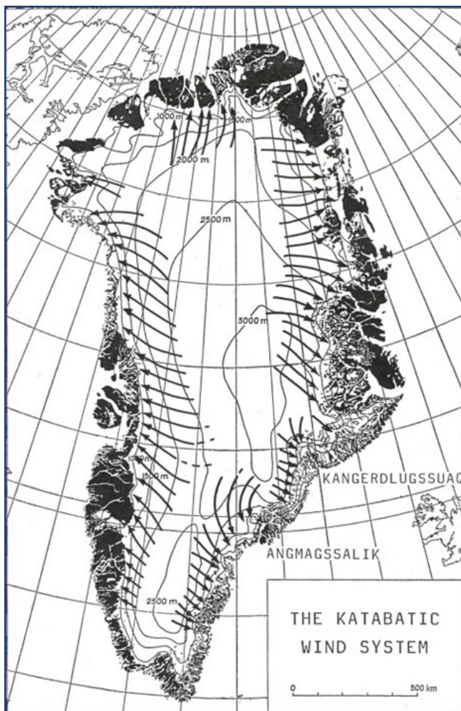
Figure 6: The katabatic wind pattern over the ice cap. The deviation from the natural fall line is due to the Earth's rotation. The pattern has been determined based on physical and thermal structures on the surface of the ice as they are seen on infrared satellite images. In the central area winds are often light. Source: Leif Rasmussen.
